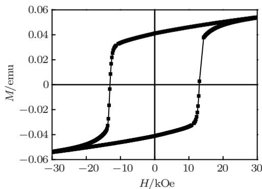
Fig. 1. Hysteresis loop for  $\text{Pr}_2\text{Fe}_{14}\text{B}$  ribbons at the temperature of 300 K.
