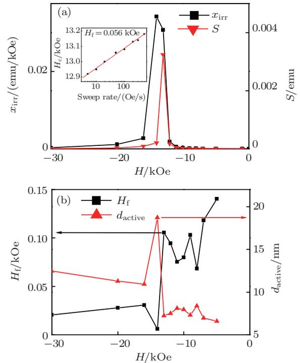
**Fig. 4.** (color online) (a) Irreversible susceptibility, viscosity coefficient, (b) fluctuation field, and activation size as functions of the applied field. The inset shows the field sweep rate dependence of coercivity for  $\text{Pr}_2\text{Fe}_{14}\text{B}$  ribbons.
