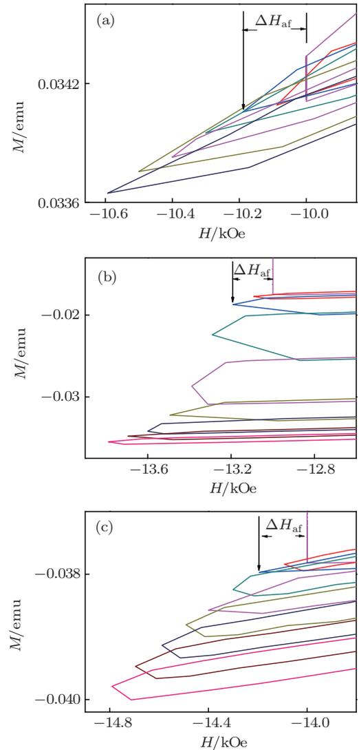
Fig. 2. (color online) Recoil loops while cycling the field to zero and back at a number of negative fields after keeping the field fixed at (a) 10 kOe, (b) 13 kOe, and (c) 14 kOe for 10 min.
