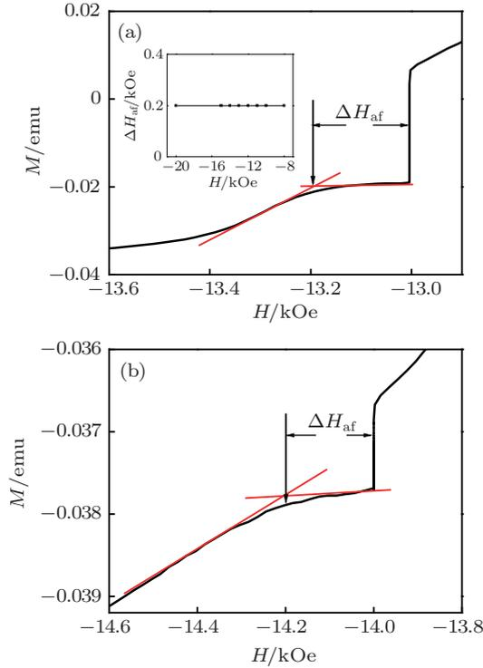
**Fig. 3.** (color online) Demagnetization curves while the field is increased at a rate of 5 Oe/s after keeping the field fixed for 10 min. The inset shows the measured aftereffect field.
