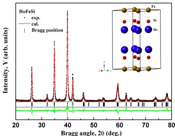
FIG. 1. The observed (dots) and calculated intensities (line drawn through the data points) of the fully refined X-ray diffraction pattern of HoFeSi compound at room temperature. The short vertical lines indicate the Bragg peak positions of the tetragonal CeFeSi-type structure. The lower curve shows the difference between the observed and calculated intensities. The inset shows the perspective view of the unit cell of HoFeSi.
