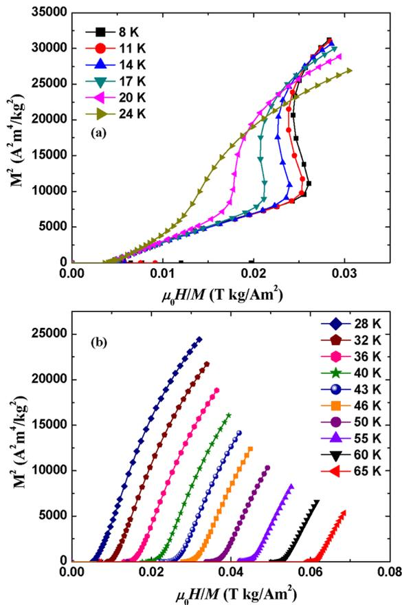
FIG. 4. (a) Arrott plots of HoFeSi compound in the temperature range of 8–24 K. (b) Arrott plots of HoFeSi compound in the temperature range of 28–65 K.
