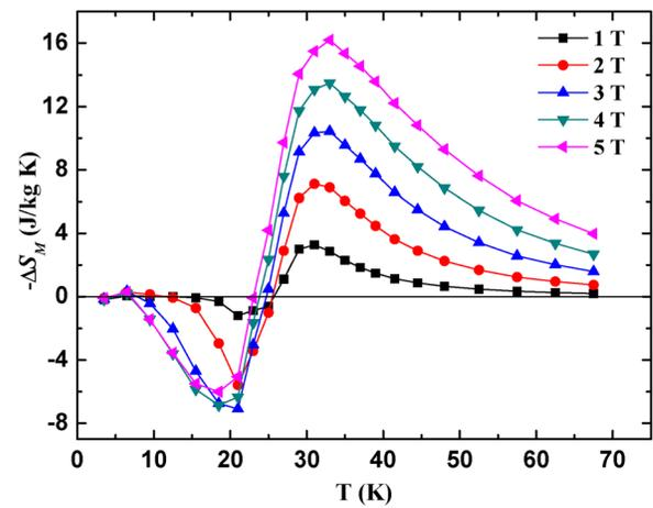
FIG. 5. Temperature dependence of magnetic entropy change  $\Delta S_M$  for HoFeSi compound under different magnetic field changes up to 5 T.
