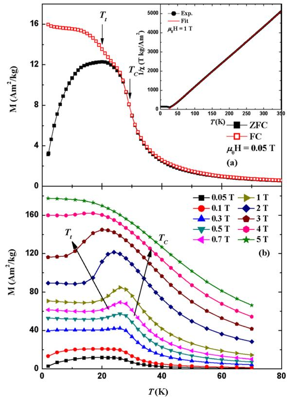
FIG. 2. (a) Temperature dependences of ZFC and FC magnetizations for HoFeSi under a magnetic field of 0.05 T. The inset shows the temperature dependence of inverse dc susceptibility ( $\chi^{-1}$ ) fitted to the Curie-Weiss law at 1 T in the temperature range of 2–350 K. (b) Temperature dependences of magnetization for HoFeSi in various magnetic fields.
