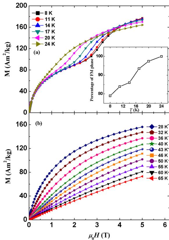
FIG. 3. (a) Magnetization isotherms of HoFeSi compound in the temperature range of 8–24 K. The inset shows the fraction of FM phase as a function of temperature estimated from magnetization isotherms. (a) Magnetization isotherms of HoFeSi compound in the temperature range of 28–65 K.
