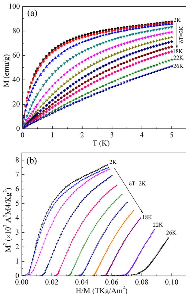
**Fig. 3.** Magnetization isotherms and the Arrott plots of TmCoAl collected in the temperature range of 2–26 K.
