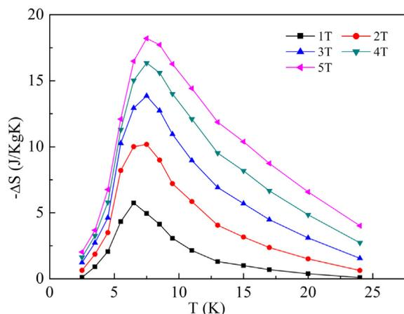
**Fig. 4.** Temperature dependences of magnetic entropy changes in TmCoAl for different magnetic field changes.
