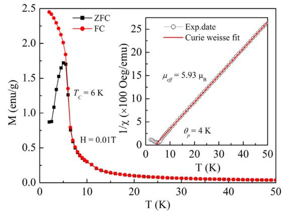
Fig. 2. Temperature dependences of ZFC and FC magnetizations of TmCoAl under the magnetic field of 0.01 T. Inset: the temperature variation of the ZFC inverse susceptibility fitted to the Curie–Weiss law.
