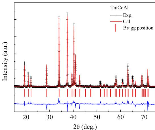
Fig. 1. Rietveld refined powder XRD patterns of TmCoAl compound at room temperature. The observed data is indicated by cross line, and the calculated profile is the straight line overlying them. The short vertical bar indicates the Bragg peak position of TmCoAl. The lower curve shows the difference between the observed and calculated intensities.
