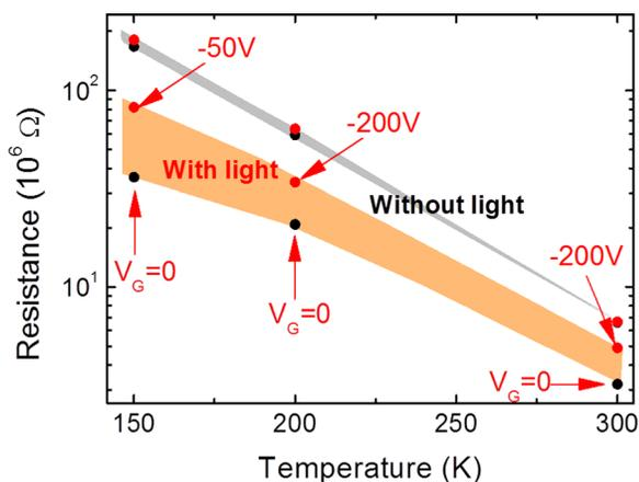
FIG. 4. A summary of the combined effects of gate field and light, obtained with a laser power of  $16.2 \text{ mW/mm}^2$  ( $\lambda = 532 \text{ nm}$ ), here only the data obtained under the  $V_G$  of 0 and  $-200 \text{ V}$  ( $|V_G| = 50 \text{ V}$  for  $T = 150 \text{ K}$  in light) are shown; the results under positive gates are similar. Orange and grey areas mark the gating effects with and without illumination, respectively.
