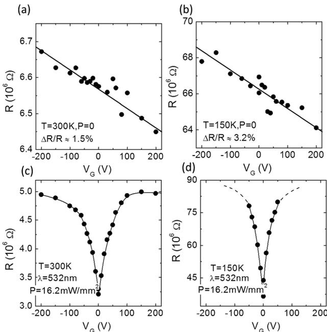
FIG. 3. (a) and (b) Resistances as functions of gate voltage, derived from the I-V curves recorded at 300 K (a) and 150 K (b). (c) and (d) Resistances as functions of gate voltage, derived from the I-V curves recorded in the presence of light at 300 K (c) and 150 K (d). Slight lines are guides for the eye.
