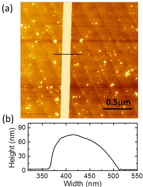
FIG. 1. (a) AFM image of the LAO nanowire grown on  $\text{TiO}_2$ -terminated STO substrate, fabricated by the technique of electrostatic spinning and post annealing. The nanowire is uniform in diameter, with a smooth surface. (b) Line profile of the nanowire, recorded along the black line marked in the image. It looks like a distorted half ellipse,  $\sim 160 \text{ nm}$  in width and  $\sim 76 \text{ nm}$  in height.
