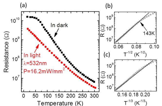
FIG. 2. (a) Resistance of the LAO nanowire grown on STO as a function of temperature, measured through the four SRO electrodes underneath LAO. Visibly light depresses the resistance by a factor up to 8. (b) Transport behavior in the form of one-dimensional variable-range hopping. (c) Transport behavior in the form of two-dimensional variable-range hopping. Combined with the results in (c) and (b) gives a better description to the transport behavior. Solid lines are guides for the eye.
