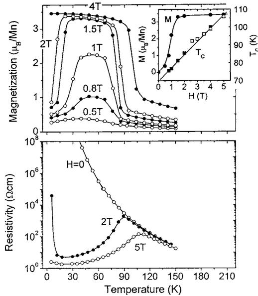
FIG. 1. Temperature-dependent magnetization of  $\text{Eu}_{0.58}\text{Sr}_{0.42}\text{MnO}_3$  measured under different magnetic fields (top panel), and the corresponding resistivity (bottom panel). Inset plot shows the variation of magnetization ( $T=45$  K) and Curie temperature with magnetic field. White squares denote the  $T_c$  determined by heat capacity. Solid lines are guides for the eye.
