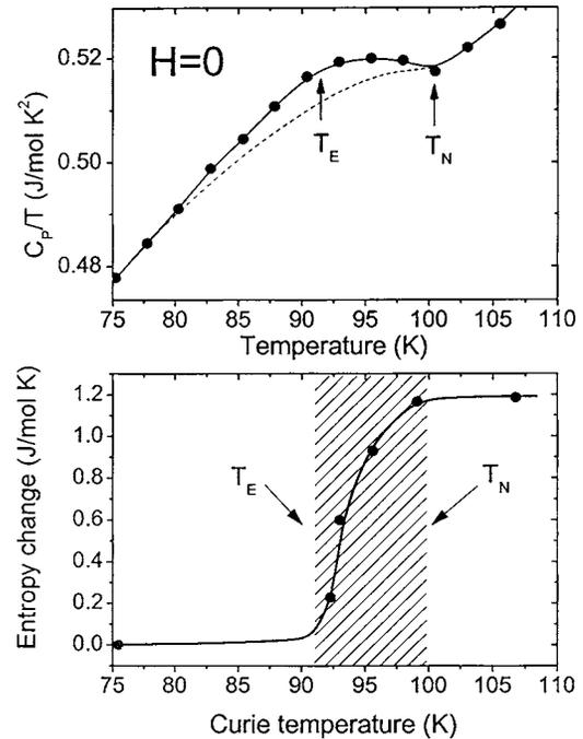
FIG. 3. Definition of the Néel temperature and the ending point for the AFM transition based on the data of heat capacity (top panel) and the magnetic entropy change as a function of Curie temperature (bottom panel). Dashed curve is the smooth background determined by a polynomial fitting. Solid lines are guides for the eye. Hatched area marks the temperature region for the AFM transition.
