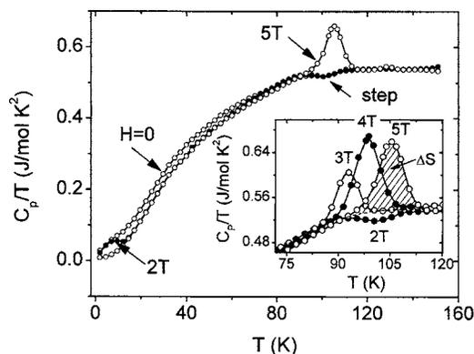
FIG. 2. Temperature-dependent heat capacity of  $\text{Eu}_{0.58}\text{Sr}_{0.42}\text{MnO}_3$  measured under selected magnetic fields. Inset plot is a close view of the heat capacity around  $T_c$ . Hatched area marks the magnetic entropy change due to the FM transition. Solid lines are guides for the eye.
