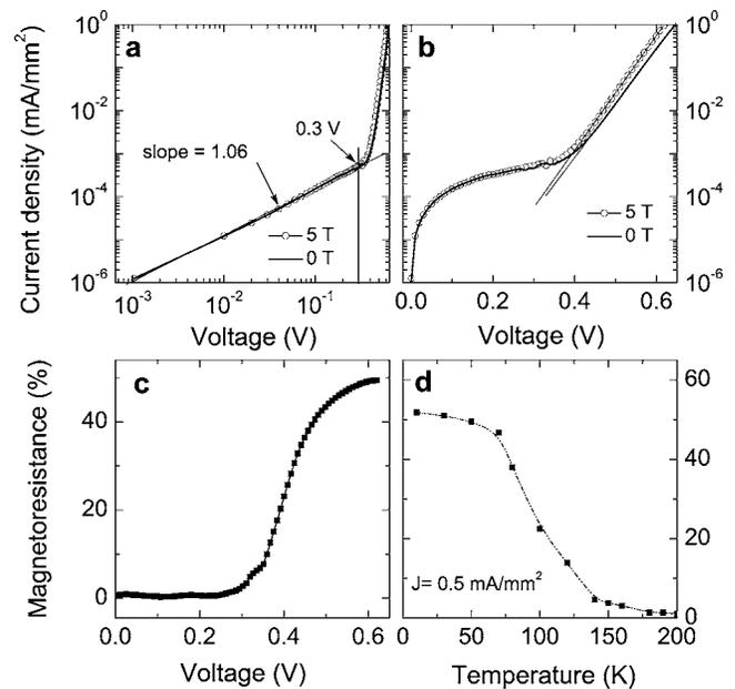
FIG. 3. (a)  $I$ - $V$  characteristics of LSMO/1% STON with and without 5 T magnetic field at 50 K, drawn in double-log coordinates. (b) Redrawing (a) in semilog coordinates. (c) MR as a function of bias at 50 K. (d) MR as a function of temperature at  $J=0.5$  mA/mm<sup>2</sup>. Thin lines are guide for eyes.
