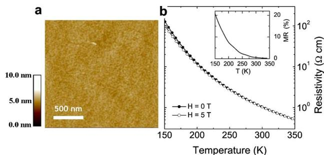
FIG. 1. (Color online) (a) AFM image of the 2 nm LSMO film. The root-mean-square roughness is  $\sim 0.24$  nm. (b) In-plane resistivity  $\rho$  as a function of temperature  $T$  for the 2 nm LSMO film grown on (001)  $\text{SrTiO}_3$  substrate. The inset shows the MR, defined as  $[\rho(0\text{ T}) - \rho(5\text{ T})] / \rho(0\text{ T})$ , of the film.
