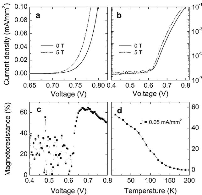
FIG. 4.  $I$ - $V$  characteristics of LSMO/0.05% STON with and without 5 T magnetic field at 10 K. (b) Redrawing (a) in semilog coordinates. (c) MR as a function of bias at 10 K. (d) MR as a function of temperature at  $J = 0.05 \text{ mA/mm}^2$ .
