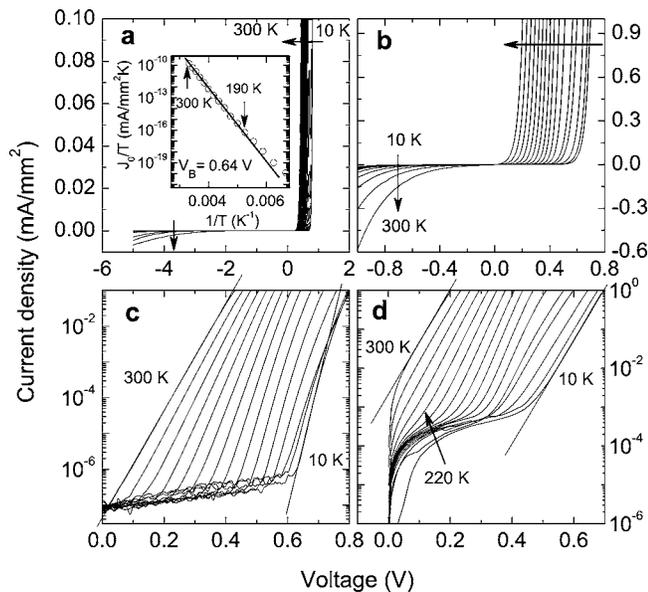
FIG. 2.  $I$ - $V$  characteristics at different temperatures for junctions (a) LSMO/0.05% STON and (b) LSMO/1% STON. In (c) and (d), we redraw the results of (a) and (b) in semilog coordinates, respectively. The inset of (a) displays saturation current as a function of reciprocal temperature, based on which the built-in potential is determined. Thin lines are guide for eyes.
