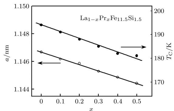
**Fig. 2.** Crystal lattice parameter and Curie temperature for the  $\text{La}_{1-x}\text{Pr}_x\text{Fe}_{11.5}\text{Si}_{1.5}$  ( $0 \leq x \leq 0.5$ ) compounds versus Pr content.
