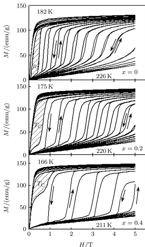
**Fig. 3.** Magnetization isotherms of the  $\text{La}_{1-x}\text{Pr}_x\text{Fe}_{11.5}\text{Si}_{1.5}$  compounds with  $x = 0, 0.2$  and  $0.4$  measured in the field-ascending and field-descending processes.
