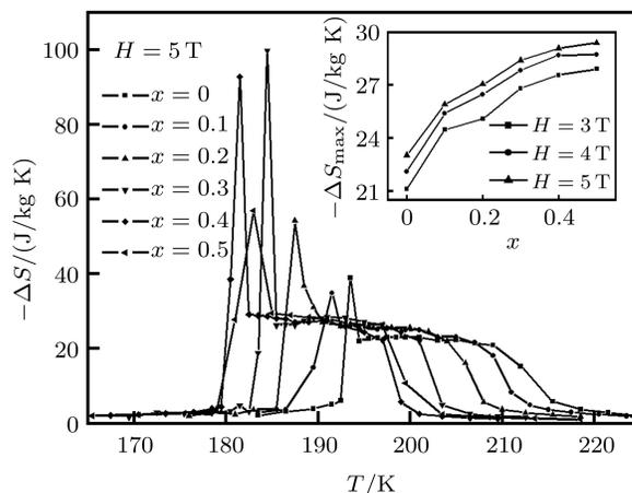
**Fig.5.** Temperature dependences of the entropy change of  $\text{La}_{1-x}\text{Pr}_x\text{Fe}_{11.5}\text{Si}_{1.5}$  ( $x = 0, 0.1, 0.2, 0.3, 0.4, 0.5$ ) compounds in magnetic fields changing from 0 to 5 T. The inset presents the magnetic entropy change as a function of Pr content.
