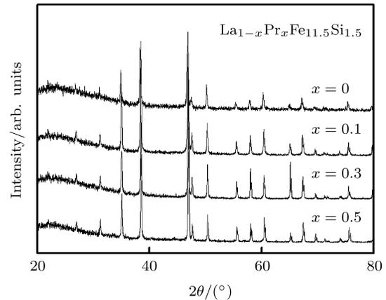
**Fig. 1.** Room-temperature powder XRD patterns of the  $\text{La}_{1-x}\text{Pr}_x\text{Fe}_{11.5}\text{Si}_{1.5}$  compounds with  $x = 0, 0.1, 0.3$  and  $0.5$ .
