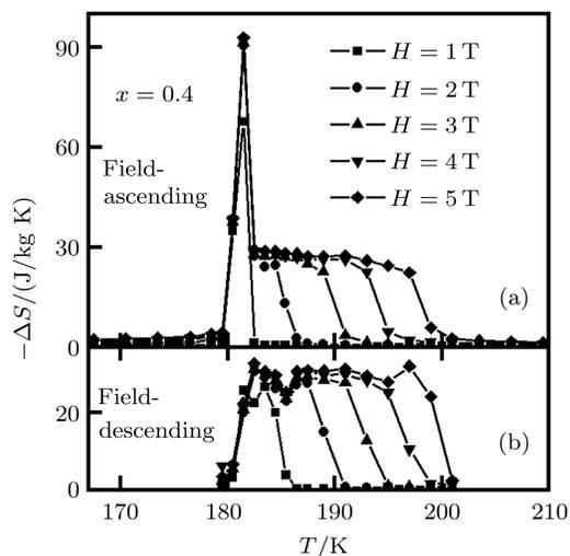
**Fig.4.** Magnetic entropy changes of  $\text{La}_{0.6}\text{Pr}_{0.4}\text{Fe}_{11.5}\text{Si}_{1.5}$  compound versus temperature based on magnetization data measured in the field-ascending (a) and field-descending (b) processes.
