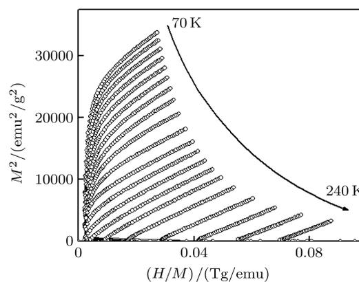
**Fig.6.** The Arrott plot of  $\text{Tb}_6\text{Co}_{1.67}\text{Si}_3$ .
