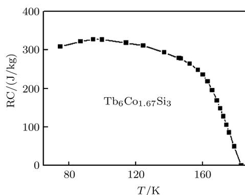
**Fig.8.** Temperature-dependent refrigerant capacity at the cold end of the refrigeration cycle for  $\text{Tb}_6\text{Co}_{1.67}\text{Si}_3$  under a maximum applied field of 5 T.
