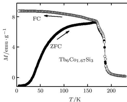
**Fig.2.** Temperature-dependent magnetization of  $\text{Tb}_6\text{Co}_{1.67}\text{Si}_3$  in zero field-cooled (ZFC) and field-cooled (FC) processes under a field of  $H = 0.01$  T.
