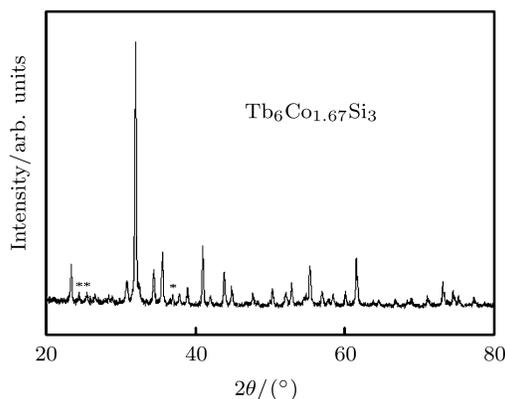
**Fig.1.** Room-temperature powder XRD patterns of  $\text{Tb}_6\text{Co}_{1.67}\text{Si}_3$  compound. The diffraction peak from impurity phase is indicated by ‘\*’.
