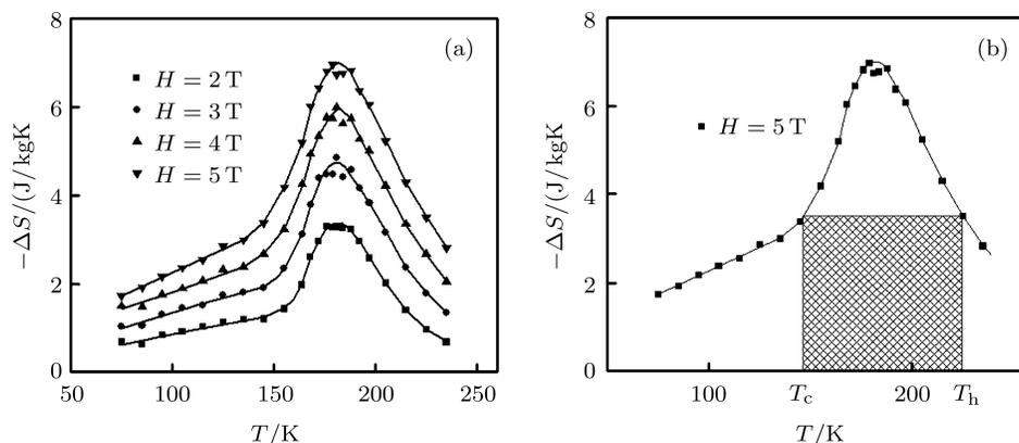
**Fig.7.** Magnetic entropy of  $\text{Tb}_6\text{Co}_{1.67}\text{Si}_3$  varying with temperature under several different magnetic fields: 2, 3, 4 and 5 T (a), and refrigerant capacity (RC) shown as the shaded area (b).
