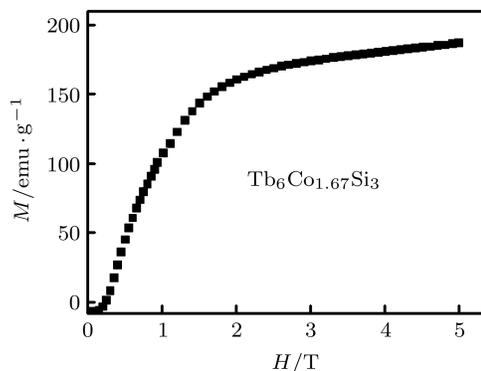
**Fig.3.** Magnetic field dependence of magnetization for  $\text{Tb}_6\text{Co}_{1.67}\text{Si}_3$  at 5 K.
