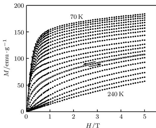
**Fig.5.** Magnetization isotherms of  $\text{Tb}_6\text{Co}_{1.67}\text{Si}_3$ , measured around the Curie temperature.
