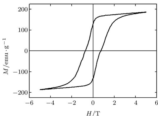
**Fig.4.** Magnetization curve for  $\text{Tb}_6\text{Co}_{1.67}\text{Si}_3$  at 5 K.
