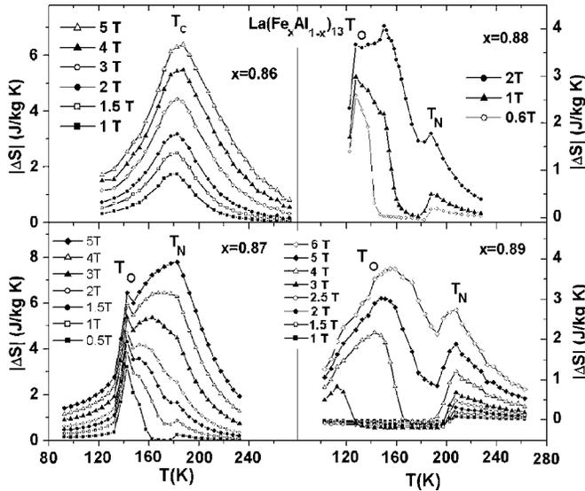
FIG. 3. Magnetic entropy change  $\Delta S$  as functions of temperature and magnetic field for  $\text{La}(\text{Fe}_x\text{Al}_{1-x})_{13}$  ( $x=0.86, 0.87, 0.88,$  and  $0.89$ ) compounds.
