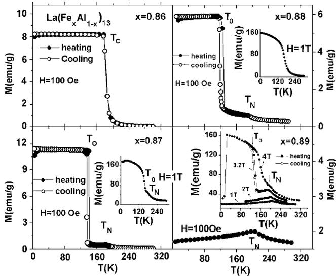
FIG. 1. Temperature dependent magnetization  $M$ - $T$  measured under 100 Oe for  $\text{La}(\text{Fe}_x\text{Al}_{1-x})_{13}$  ( $x=0.86, 0.87, 0.88,$  and  $0.89$ ) compounds. Insets are  $M$ - $T$  curves under relatively high fields for the corresponding samples.
