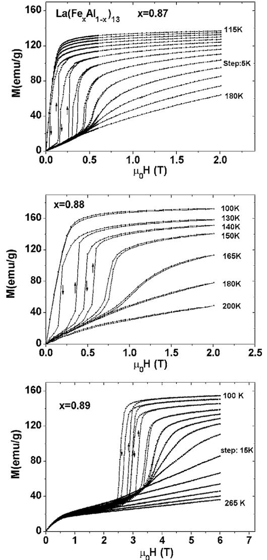
FIG. 2. Magnetization isotherms  $M$ - $H$  for  $\text{La}(\text{Fe}_x\text{Al}_{1-x})_{13}$  ( $x=0.87, 0.88,$  and  $0.89$ ) compounds measured upon magnetic field increase and decrease.
