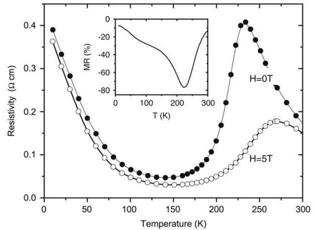
Fig. 1. Temperature dependence of the in-plane resistivities for a  $La_{0.7}Ce_{0.3}MnO_3$  film, measured with  $H = 0$  and  $H = 5$  T field. In the inset is the temperature dependence of MR  $[\rho(5 \text{ T})/\rho(0 \text{ T}) - 1]$  for the film.
