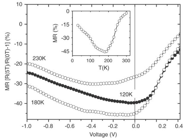
Fig. 5. Bias dependence of MR [ $R(5\text{ T})/R(0\text{ T}) - 1$ ] for the  $\text{La}_{0.7}\text{Ce}_{0.3}\text{MnO}_3$  / 1 wt% Nb-doped  $\text{SrTiO}_3$  junction at various temperatures. At each temperature, the maximal value of MR appears near 0 V bias. In the inset is the temperature dependence of the maximal MR for the junction.
