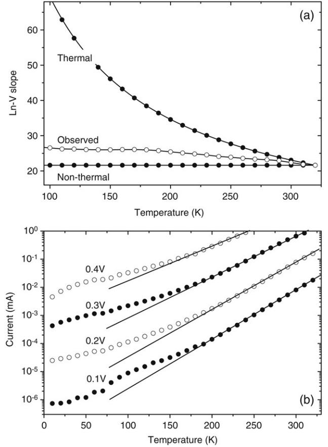
Fig. 3. (a) Temperature dependence of the slopes of  $\ln I$ - $V$  curves for the thermal and non-thermal processes. Experimental results are shown for comparison. (b) Temperature dependence of current at different bias voltages. Solid lines are guides for the eye.
