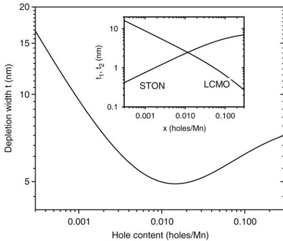
Fig. 4. Depletion width as a function of mobile hole content in the LCMO film. The inset shows the depletion widths of LCMO and STON, respectively.
