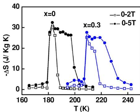
FIG. 5. (Color online) Temperature dependence of the magnetic entropy change of  $\text{La}_{0.5}\text{Pr}_{0.5}\text{Fe}_{11.5}\text{Si}_{1.5}\text{C}_x$  compounds with  $x=0$  and  $0.3$  for magnetic field changes from  $0$  to  $2$  T and from  $0$  to  $5$  T.
