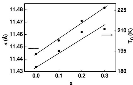
FIG. 2. Crystal lattice parameter and Curie temperature for  $\text{La}_{0.5}\text{Pr}_{0.5}\text{Fe}_{11.5}\text{Si}_{1.5}\text{C}_x$  ( $0 \leq x \leq 0.3$ ) compounds as functions of carbon concentration.
