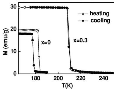
FIG. 1. Thermomagnetization curves for  $\text{La}_{0.5}\text{Pr}_{0.5}\text{Fe}_{11.5}\text{Si}_{1.5}\text{C}_x$  compounds with  $x=0$  and  $0.3$  measured during heating and cooling under a magnetic field of  $0.05$  T.
