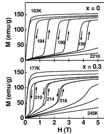
FIG. 3. Magnetization isotherms of  $\text{La}_{0.5}\text{Pr}_{0.5}\text{Fe}_{11.5}\text{Si}_{1.5}\text{C}_x$  compounds with  $x=0$  and  $0.3$  measured under increasing and decreasing fields in a range of temperatures around the Curie temperature.
