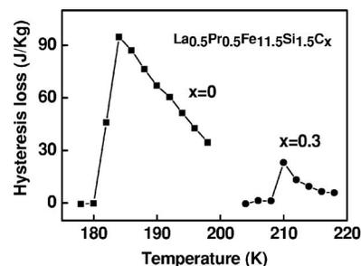
FIG. 4. Temperature dependence of hysteresis loss of  $\text{La}_{0.5}\text{Pr}_{0.5}\text{Fe}_{11.5}\text{Si}_{1.5}\text{C}_x$  compounds with  $x=0$  and  $0.3$ .
