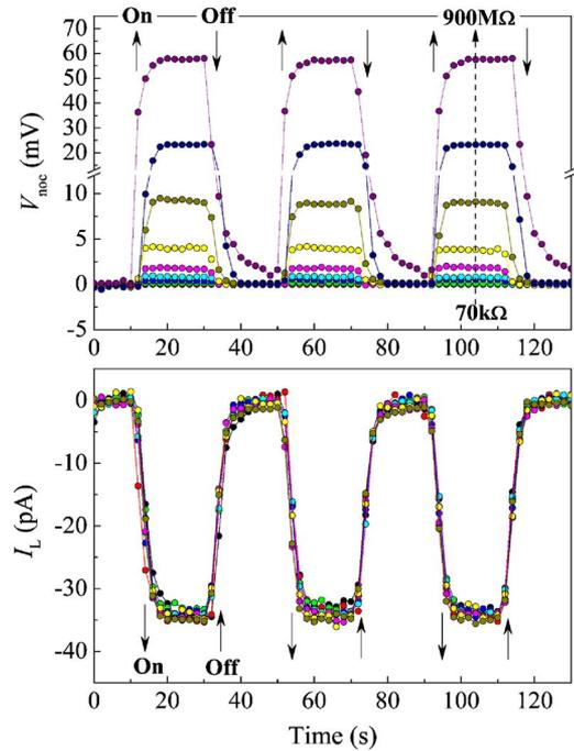
FIG. 2. (Color online) Photovoltage (a) and photocurrent (b) produced by light illumination for the Au/STON junction in different resistance states. The resistance ranged from 70 k $\Omega$  to 900 M $\Omega$ . Short arrows specify the time for the light on and light off.
