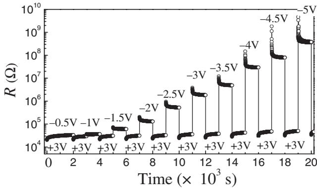
FIG. 1. Resistances of the Au/STON junction triggered by electric pulses with different polarities and amplitudes. Pulse width was fixed at 1 ms. Readout voltage is 0.05 V.
