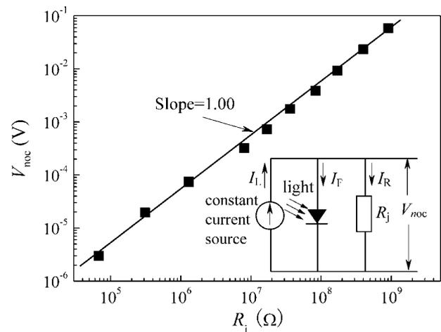
FIG. 3. Open-circuit photovoltages ( $V_{\text{noc}}$ ) as functions of junction resistance. The slope of the fit line is 1.00, demonstrating the linear resistance dependence of  $V_{\text{noc}}$ .  $I_L = 34$  pA, directly calculated from the intercept of fit line with the  $V_{\text{noc}}$ -axis. Inset plot: the equivalent circuit consists of a diode in parallel with a resistor, modeling the photoelectronic processes in the junction.
