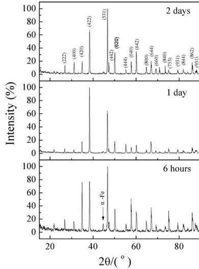
FIG. 1. X-ray diffraction patterns of  $\text{LaFe}_{10.8}\text{Co}_{0.7}\text{Si}_{1.5}\text{C}_{0.2}$  compounds (annealing for 3 h, 6 h, 1 day, and 2 days).
