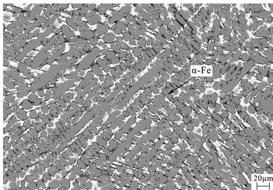
FIG. 2. Backscattered SEM micrographs of as-cast sample.
