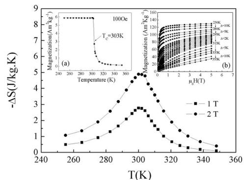
FIG. 4. Magnetic entropy changes of  $\text{LaFe}_{10.8}\text{Co}_{0.7}\text{Si}_{1.5}\text{C}_{0.2}$  compound annealed for 2 days. (a) MT curve of  $\text{LaFe}_{10.8}\text{Co}_{0.7}\text{Si}_{1.5}\text{C}_{0.2}$  compound. (b) Isothermal magnetization of  $\text{LaFe}_{10.8}\text{Co}_{0.7}\text{Si}_{1.5}\text{C}_{0.2}$  compound.
