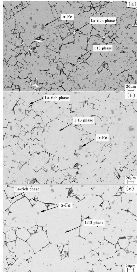
FIG. 3. Backscattered SEM micrographs of  $\text{LaFe}_{10.8}\text{Co}_{0.7}\text{Si}_{1.5}\text{C}_{0.2}$  compound after being annealed at 1373 K at different times (a) 6 h, (b) 1 day, and (c) 2 days.
