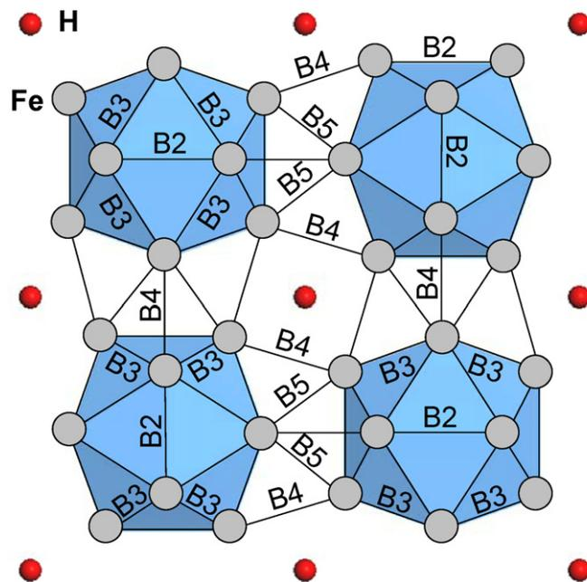
**Fig. 6.** A schematic diagram for the atomic structure of  $\text{LaFe}_{13}\text{H}_3$  (La is omitted for clarity).
