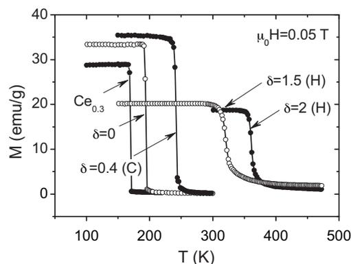
**Fig. 7.** Temperature dependence of magnetization measured under the field of 0.05 T for the  $\text{La}_{0.7}\text{Ce}_{0.3}\text{Fe}_{11.5}\text{Si}_{1.5}$ ,  $\text{LaFe}_{11.5}\text{Si}_{1.5}\text{H}_\delta$  ( $\delta=0, 1.5$ , and 2.0) and  $\text{LaFe}_{11.5}\text{Si}_{1.5}\text{C}_\delta$  ( $\delta=0.4$ ) compounds.
