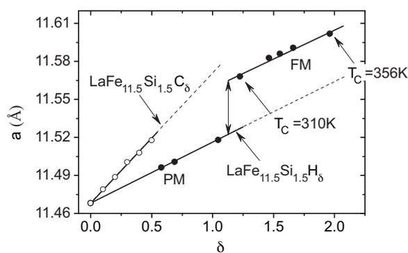
**Fig. 2.** Lattice constant as a function of the content of interstitial atoms for the  $\text{LaFe}_{11.5}\text{Si}_{1.5}\text{H}_\delta$  hydrides and  $\text{LaFe}_{11.5}\text{Si}_{1.5}\text{C}_\delta$  carbides. Solid and dashed lines are guides for the eye.
