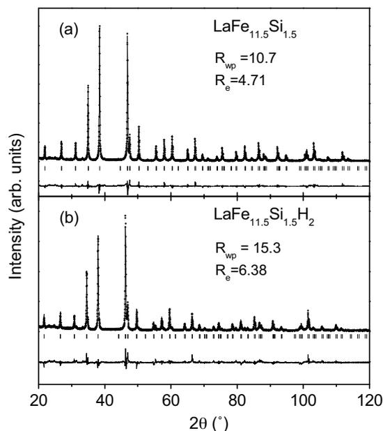
**Fig. 1.** Observed (crosses) and calculated (solid lines) XRD patterns of the  $\text{LaFe}_{11.5}\text{Si}_{1.5}$  and  $\text{LaFe}_{11.5}\text{Si}_{1.5}\text{H}_2$  compounds. The lowest curve shows the difference between observed and calculated patterns. Vertical bars show the positions of Bragg reflections.
