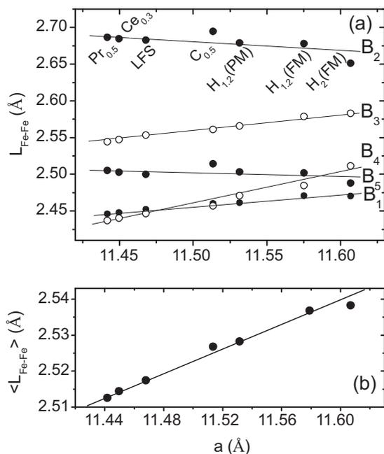
**Fig. 5.** Bond length (a) and average bond length (b) as functions of lattice constant for  $\text{La}_{0.7}\text{Ce}_{0.3}\text{Fe}_{11.5}\text{Si}_{1.5}$ ,  $\text{LaFe}_{11.5}\text{Si}_{1.5}\text{H}_\delta$  ( $\delta=0, 1.2, 2$ ) and  $\text{LaFe}_{11.5}\text{Si}_{1.5}\text{C}_{0.5}$  compounds. Results of  $\text{La}_{0.5}\text{Pr}_{0.5}\text{Fe}_{11.5}\text{Si}_{1.5}$  were also shown for comparison. Solid lines are guides for the eye.
