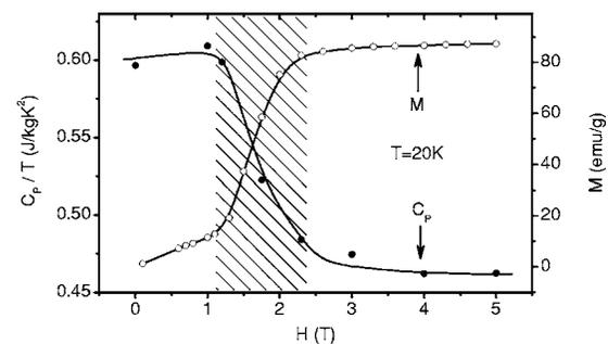
FIG. 4. Heat capacity and isothermal magnetization as functions of magnetic field measured at a fixed temperature of  $T=20$  K. The hatched area marks the AFM-FM transition. The solid lines are guides for the eyes.
