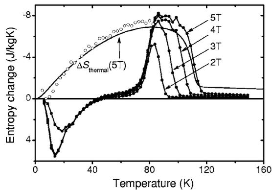
FIG. 2. Entropy changes in  $\text{Eu}_{0.55}\text{Sr}_{0.45}\text{MnO}_3$  determined by Maxwell relation (solid symbols), specific heat (solid lines), and the extra two terms plus the Maxwell result (open circles), respectively.
