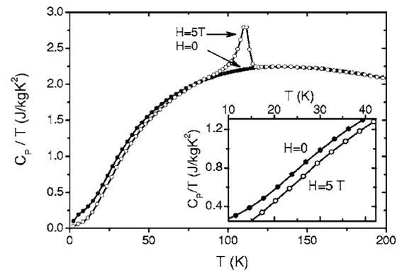
FIG. 3. Heat capacity of  $\text{Eu}_{0.55}\text{Sr}_{0.45}\text{MnO}_3$  measured under the fields of  $H=0$  and 5 T. The inset plot is a close view of the heat capacity in the low temperature range.
