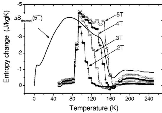
FIG. 5. Entropy changes in  $\text{La}_{0.27}\text{Nd}_{0.40}\text{Ca}_{0.33}\text{MnO}_3$  determined by Maxwell relation (solid symbols) and heat capacity (solid lines), respectively.
