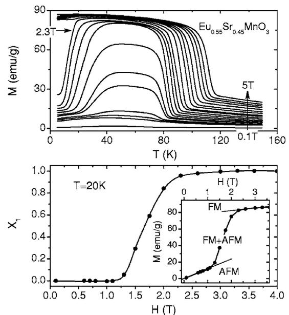
FIG. 1. Thermal magnetization of  $\text{Eu}_{0.55}\text{Sr}_{0.45}\text{MnO}_3$  measured under different magnetic fields (top panel) and the proportion of the FM phase ( $X_1$ ) as a function of magnetic field at a selected temperature of 20 K (bottom panel). Bottom inset shows the corresponding isothermal magnetization curve for  $T=20$  K. The solid lines are guides for the eyes.
