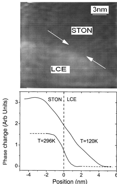
FIG. 2. (Top panel) Reconstructed phase image from the hologram taken at 296 K. (Bottom panel) Phase profiles showing the change of the electrostatic potential across the LCE/STON interface obtained at 120 and 296 K, respectively. Dark and bright areas correspond to high and low electron phase, respectively. Arrows and dashed line mark the LCE/STON interface.
