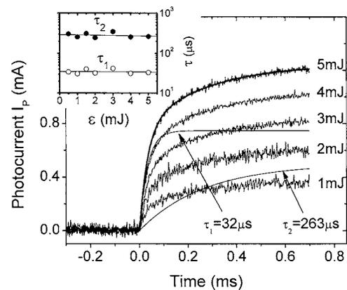
FIG. 3. Photocurrent as a function of time measured under different pulse intensities. Results of curve-fitting based on two exponentials are also provided for  $\epsilon = 5$  mJ (thick and smooth curve). Thin curves represent the two distinctive processes for the pulse energy of 5 mJ. Inset plot shows the time constants against pulse intensity.
