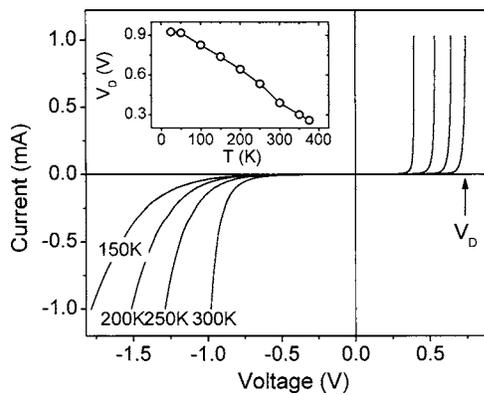
FIG. 1. Selected current-voltage curves measured at different temperatures below 300 K. Inset is a plot of diffusion voltage (marked by the arrow in the main figure) as a function of temperature.
