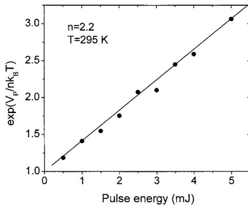
FIG. 4. Photovoltage as a function of pulse intensity measured at ambient temperature. Solid line is a guide for the eye.
